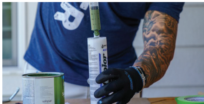
Paint injected directly into the cartridge — two-step mixing, then 30 minutes for the thickener to fully set before application.
