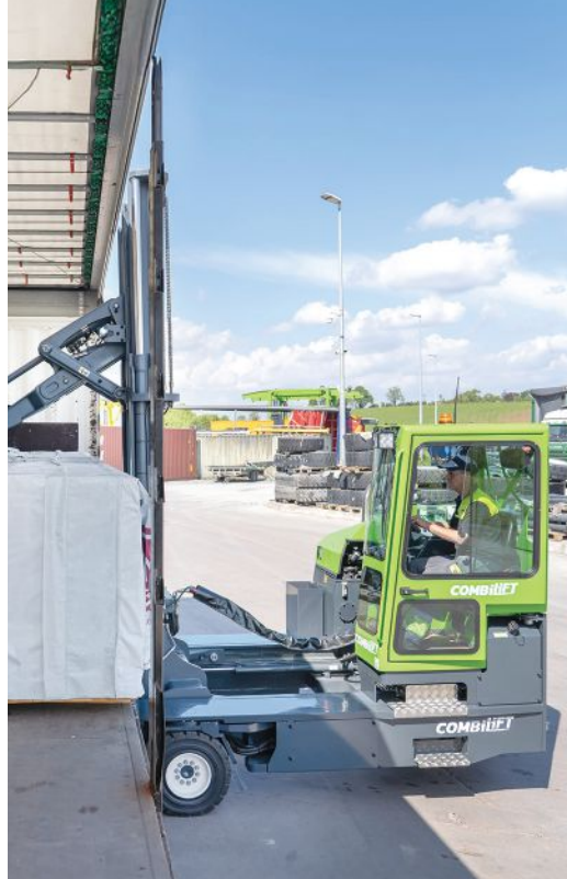
Combilift’s Load Xtender, a new pantograph-style load extender that allows full truck or container loading from one side only, is designed as a solution for businesses operating in restricted loading areas, where double-side access to trailers is not possible, or where space is limited.
