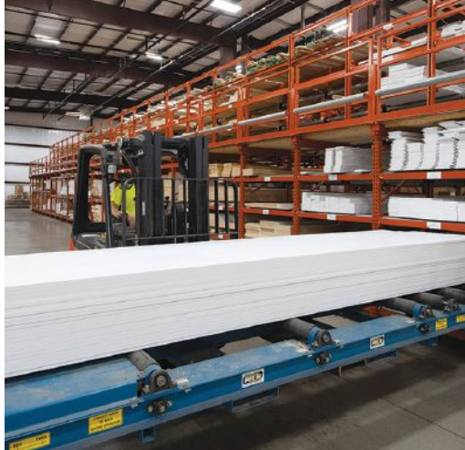
CT Darnell’s Power Bin is a battery-operated loader deck which automatically loads materials into pigeonhole bins. Loading reportedly takes approximately one minute, which significantly decreases labor costs.
