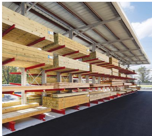
As CT Darnell explains, I-beam cantilever racks can function as the building blocks for T-sheds, L-sheds and drive-thru buildings or as a stand-alone, multi-level, high-density storage system for long-length materials such as engineered wood products.
