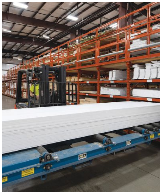
The Sunbelt Rack Power Bin handles and stores lumber, siding, moulding, composite decking, and other materials. According to the manufacturer, a battery-operated loader places material into pigeonhole bins equipped with heavy-duty rollers in approximately one minute. The bins can be customized and configured to specific needs.
