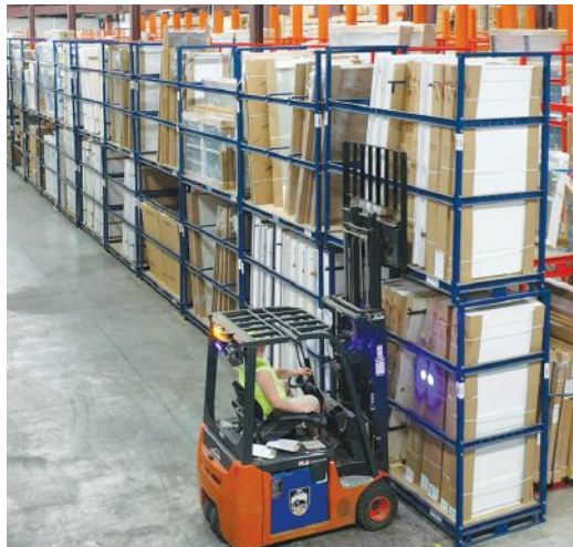
LEFT: Sunbelt Rack’s millwork stack racks are movable, stackable storage systems for windows, doors, and other products. Because they’re movable, you can load millwork onto them directly at the assembly area and then move them to a warehouse or staging area. According to Sunbelt, they can be stacked up to three racks high, allowing for high-density storage and saving warehouse floor space.
