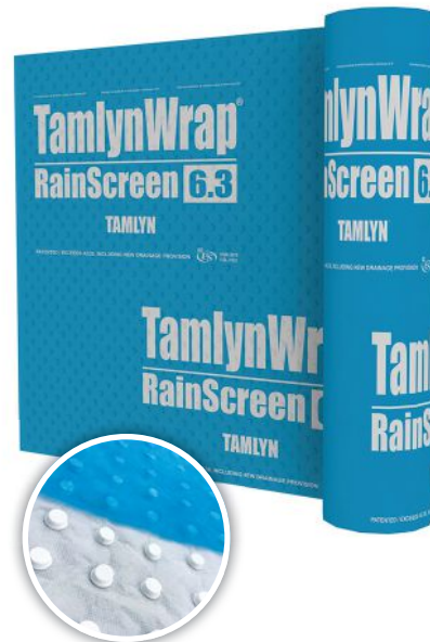
TamlynWrap RainScreen is a multi-layer water management system intended for use over existing water-resistant barrier or coated sheathing systems. According to Tamlyn, it’s ideal for use behind stucco, stone, fiber cement board and metal panels. The 6.3 mm (1/4”) or 10.1 mm (3/8”) thick cavity spacers are non-compressible and can act as furring strips to promote enhanced drainage and drying capacity with improved installation efficiency.
