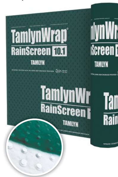
TamlynWrap RainScreen is a multi-layer water management system intended for use over existing water-resistant barrier or coated sheathing systems. According to Tamlyn, it’s ideal for use behind stucco, stone, fiber cement board and metal panels. The 6.3 mm (1/4”) or 10.1 mm (3/8”) thick cavity spacers are non-compressible and can act as furring strips to promote enhanced drainage and drying capacity with improved installation efficiency.
