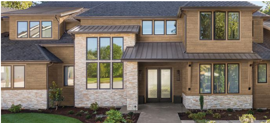
ABOVE: The UFP-Edge Thermally Modified Wood Cladding is made from a process that uses heat and steam to stabilize the wood without the use of chemicals. According to UFP, this process makes it less vulnerable to shrinking and seasonal expansion and contraction.
