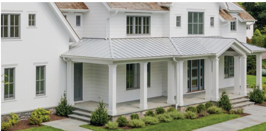
BELOW: Boral's TruExterior Siding Craftsman Collection includes seven historically and architecturally accurate profiles designed to replicate the look of traditional wood siding. It is made with a proprietary blend of fly ash and polymers and requires no sealing of ends or cuts in the field, can be used in ground-contact applications, and can be painted any color, including dark hues.
