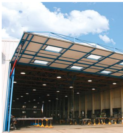
RIGHT: New from Schweiss Doors is its Superstructure doorframe for bifold and hydraulic doors. According to the manufacturer, this one-of-a-kind tripod leg stand-alone design transfers the door weight to the footings that support the hydraulic door, eliminating the need for additional side columns from the building manufacturer or a need for the building manufacturer to incorporate a building truss or building header to support the hydraulic door on the structure.
