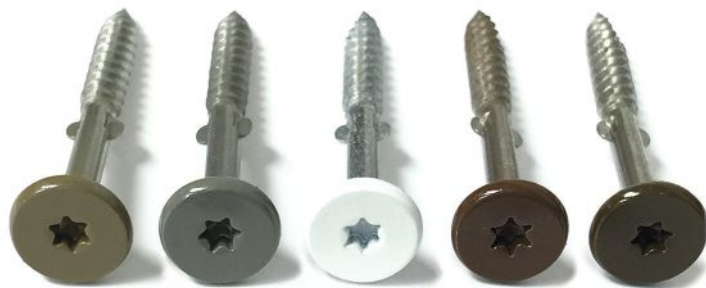
BELOW: Sure Drive's new Sure-Hold one-step stainless steel fastener for installing composite fascia board has cutting wings built to create an oversized hole that allows for expansion and contraction, while an oversized head increases bearing surface and maximum hole coverage.
