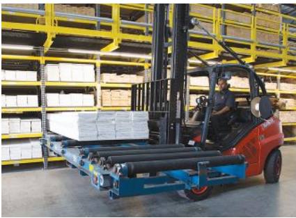
The Sunbelt Rack Power Bin handles and stores lumber, siding, moulding, composite decking and other materials. According to the manufacturer, a battery-operated loader places material into pigeonhole bins equipped with heavy-duty rollers in approximately one minute. The bins can be customized and configured to specific needs.
