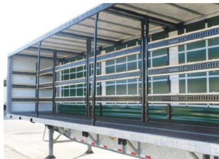
RIGHT: Center-Line’s curtain-side trailers allow materials to be loaded to evenly distribute weight rather than by destination, the manufacturer says. As well, because forklifts have greater access, the trailers are faster to load and unload, and they eliminate the need for the driver to climb on the load or tarp it for protection during delivery.
