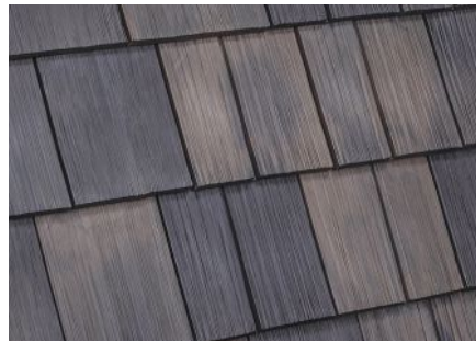
DaVinci Roofscapes' Select Shake multi-width tiles mimic the look of cedar shake. Available in 8" and 10" widths, each tile is 22" long and has a 5/8" thickness. According to DaVinci, the unique tile design allows for faster installation than previous DaVinci single- and multi-width products.
