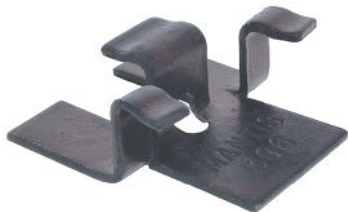
ABOVE: The Mantis Clip hidden deck fastener is described as the only product that features a base that the deck board actually rests on, instead of simply clamping the board down to the joist. This base is designed to allow for airflow that lets the joist frame dry out faster, making it last longer.
