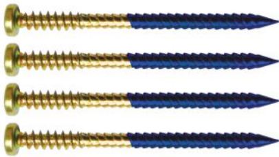
ABOVE: Fasco's new SubLoc PRO SCRAIL are for use as a substitute for 8D and 10D common nails in OSB and Plywood WSP horizontal diaphragms for resisting wind and seismic forces. The fasteners are also permitted to be used as a substitute for 8D or 10D common nails in prescriptive construction of WSP diaphragms in accordance with the IRC for maximum 15/32" thick and 19/32" thick diaphragms, respectively.
