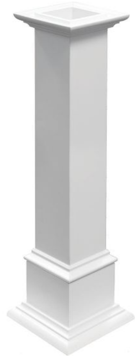
ABOVE: Boral Building Products' Kleer brand has added a 10" post wrap to its line of KLEERWrap porch and column wraps. KLEERWrap post wraps are simple to install with just one person. Each wrap comes with three sides preassembled; the installer applies adhesive to the joints of the three-sided piece and secures it around the wood post, then "snaps" the fourth side into place and fastens.
