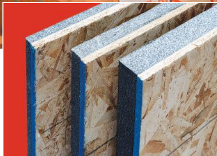
Universal Forest Products' ThermalStar One insulating structural sheathing combines four layers in one application that according to the manufacturer provides a strong, stiff, nailable structural layer with segment leading shear value, graphite enhanced rigid insulation in three thicknesses/R-Values, and an integral taped WRB/air barrier layer.
