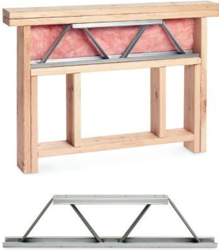
Rhino Engineered Steel Headers are designed for a header space to be fully insulated, which provides a thermal break and eliminates the header area as part of the thermal heat-loss calculation. The patent-pending product is lightweight, easy to handle and install, and won't twist, crack or warp like wood headers.
